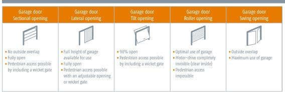
The opening system depends on the layout of your garage entrance or gate: clearance available inside and possible overlap outside.
